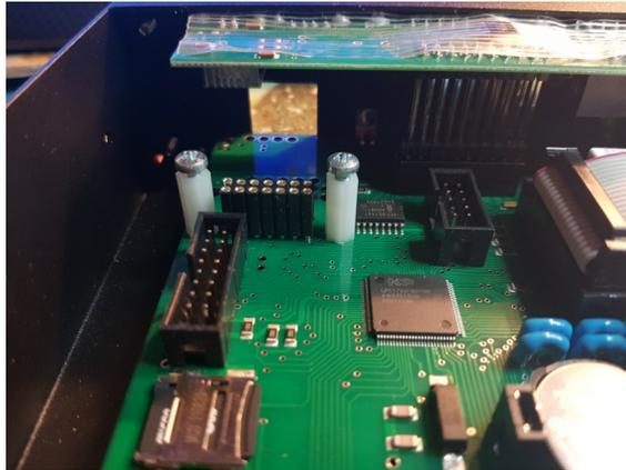
remove the two screws and the 10 pin extension bar from the photo above as shown in the photo below.
