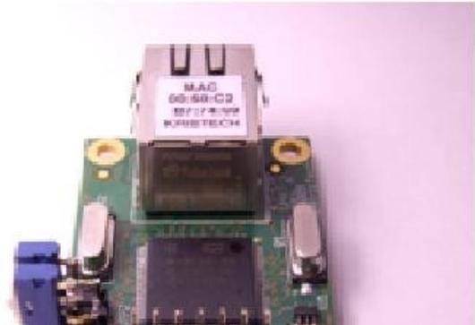
Step 2: Remove the top cover of the MD-01/02 controller. Locate the area of the Motherboard near the Ethernet connector. Remove the two screws from the standoffs.
