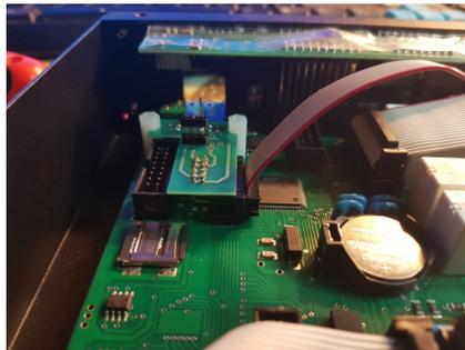
Connect the connection cable to the Mount Board as shown above and install it on the motherboard as shown.
